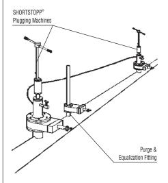
TDW SHORTSTOPP® Purge & Equalization Fittings are used for blowdown of the isolated pipe section following a double SHORTSTOPP® operation.
