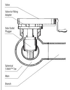
The SHORTSTOPP® 275 system's Side Outlet Plugger is used with Spherical 3-WAY™ Tees to plug the tapped hole in a main. It forms a pressure-tight seal that simultaneously allows flow to continue in the main while preventing it from escaping into the side outlet. This permits maintenance work on the branch line without interruption of flow in the main line.
