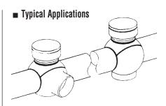
The bottom half of the Spherical 3-WAY™ Tee can be turned for either a side or bottom\* outlet as illustrated. The tee can also be installed
