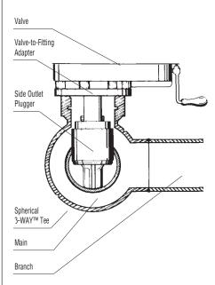
The SHORTSTOPP® 275 system's Side Outlet Plugger is used with Spherical 3-WAY™ Tees to plug the tapped hole in a main. It forms a pressure-tight seal that simultaneously allows flow to continue in the main while preventing it from escaping into the side outlet. This permits maintenance work on the branch line without interruption of
