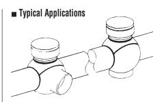
The bottom half of the Spherical 3-WAY™ Tee can be turned for either a side or bottom\* outlet as illustrated. The tee also can be installed
