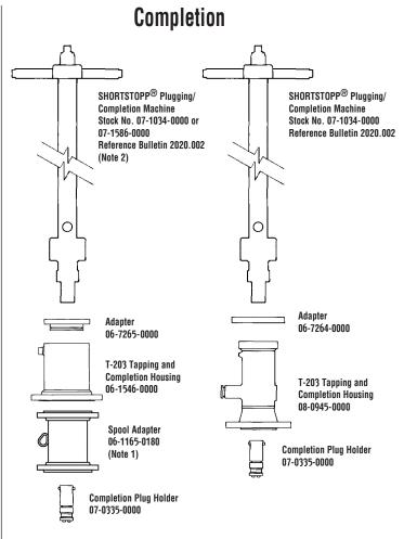
■ Note 1: 12-inch Spool Adapter required to set 12-inch SHORTPLUG<sup>TM</sup> with Guide Bars in SHORTSTOPP Type II 3-Way<sup>TM</sup> Tee fittings using the 06-1546-0000 Adapter and 07-1586-0000 Completion Machine
