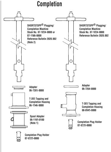
■ Note 1: 12-inch Spool Adapter required to set 10-inch SHORTPLUG™ with Guide Bars in SHORTSTOPP Type II 3-Way™ Tee fittings using the 06-1546-0000 Adapter and 07-1586-0000 Completion Machine
