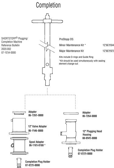
Note 1: \*12-inch Spool Adapter required to set 10-inch SHORTPLUG™ with Guide Bars in SHORTSTOPP Type II 3-Way™ Tee fittings using the 06-1546-0000 Adapter and 07-1586-0000 Completion Machine
